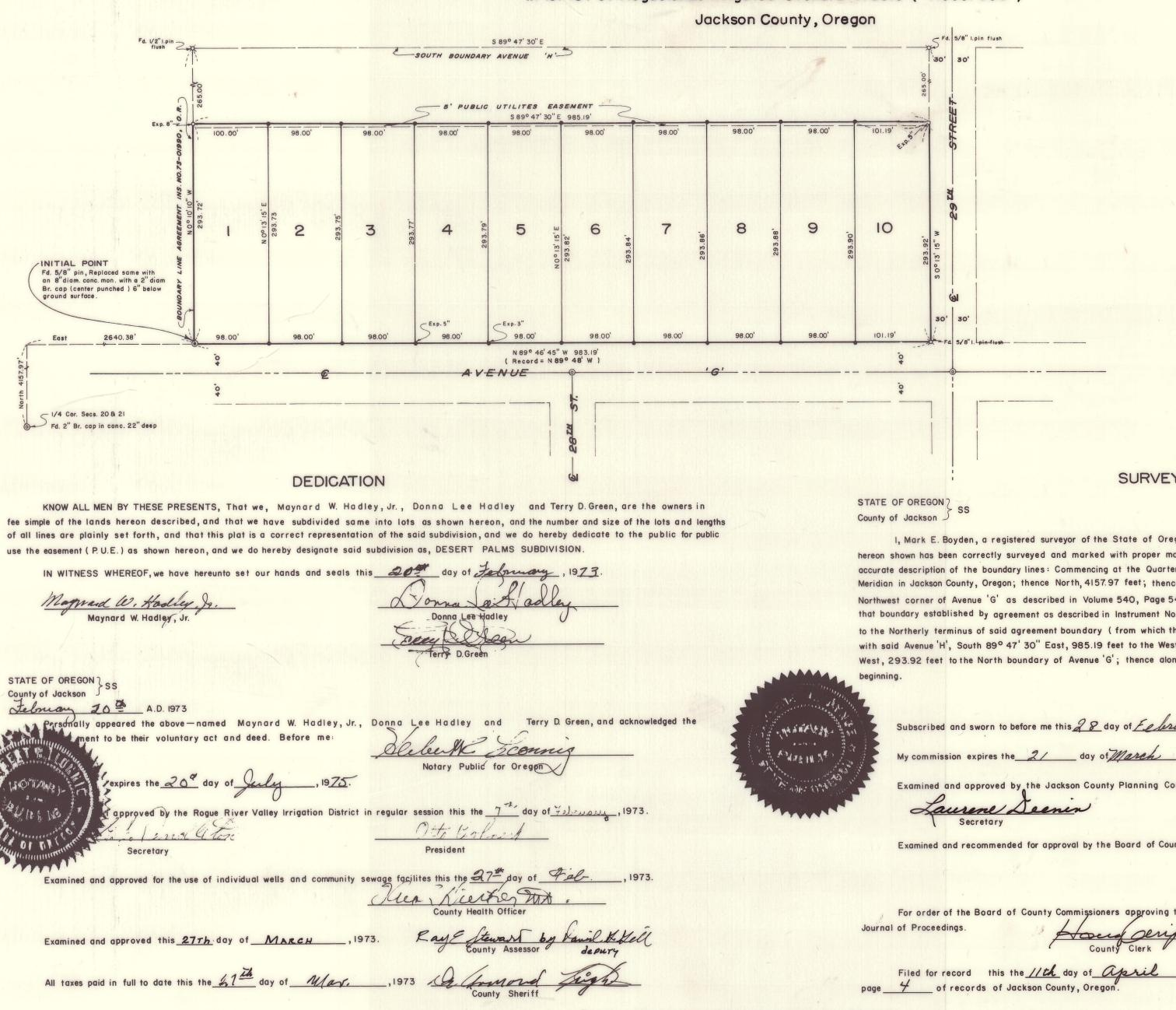
SCALE |"= 100" BASIS OF BEARINGS CASCADE VILLAGE, UNIT NO. 3 (RECORDED) Rotated clockwise 0° 00' 40" FOUND MONUMENT AS INDICATED FOUND BR. DISK IN CONC. SET 3/4" x 24" IRON PIN FLUSH UNLESS OTHERWISE INDICATED O SET 3/4" x 30" IRON PIN FLUSH UNLESS
