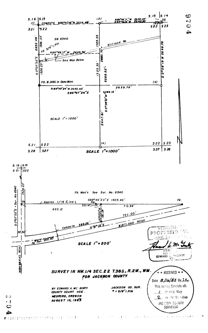
KIRTLAND ROAD: Being a road 40 feet in width on each side of the centerline. By utilizing monuments found and shown on Survey No. 6540 and the recovery of a 5/8 inch iron pin on the centerline PI, established the northerly line of Kirtland Road. (Note, there is apparently some small discrepancy in the curve data of record possible field measurements and for simplicity only, shown record semi tangent distance.)
