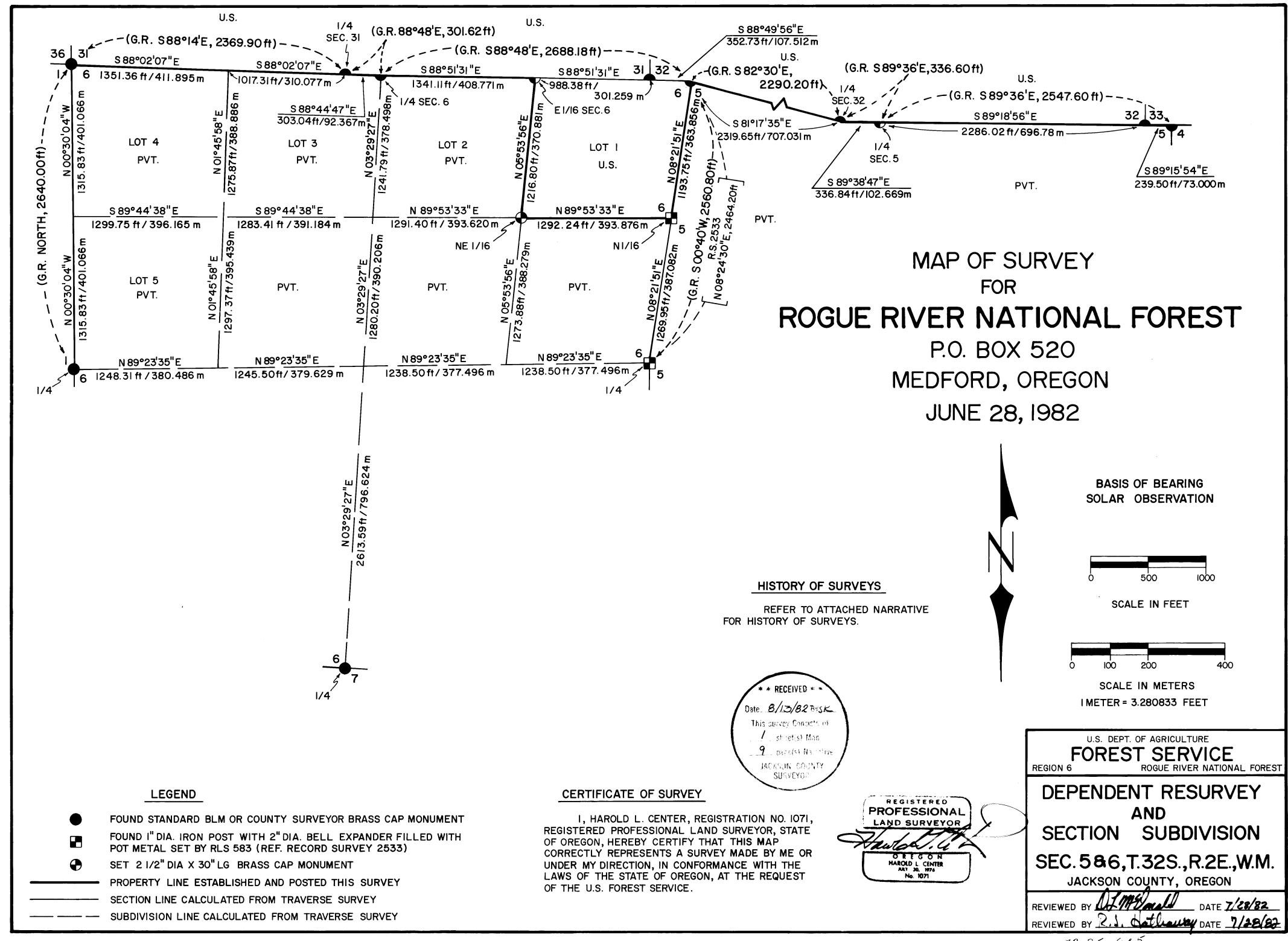
At the corner point I set a  $2\frac{1}{2}$ -inch diameter by 30-inch long galvanized iron post with a  $2\frac{1}{2}$ -inch diameter brass cap marked:
