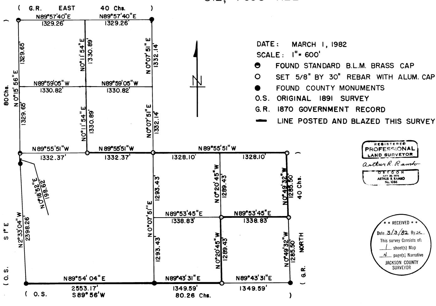
South one-sixteenth corner common to Section 12 Township 33 South Range 2 East and Section 7 Township 33 South Range 1 East. At the corner location I set a 5/8 by 30" rebar with a  $1\frac{1}{2}$  inch dia. aluminum cap marked:
