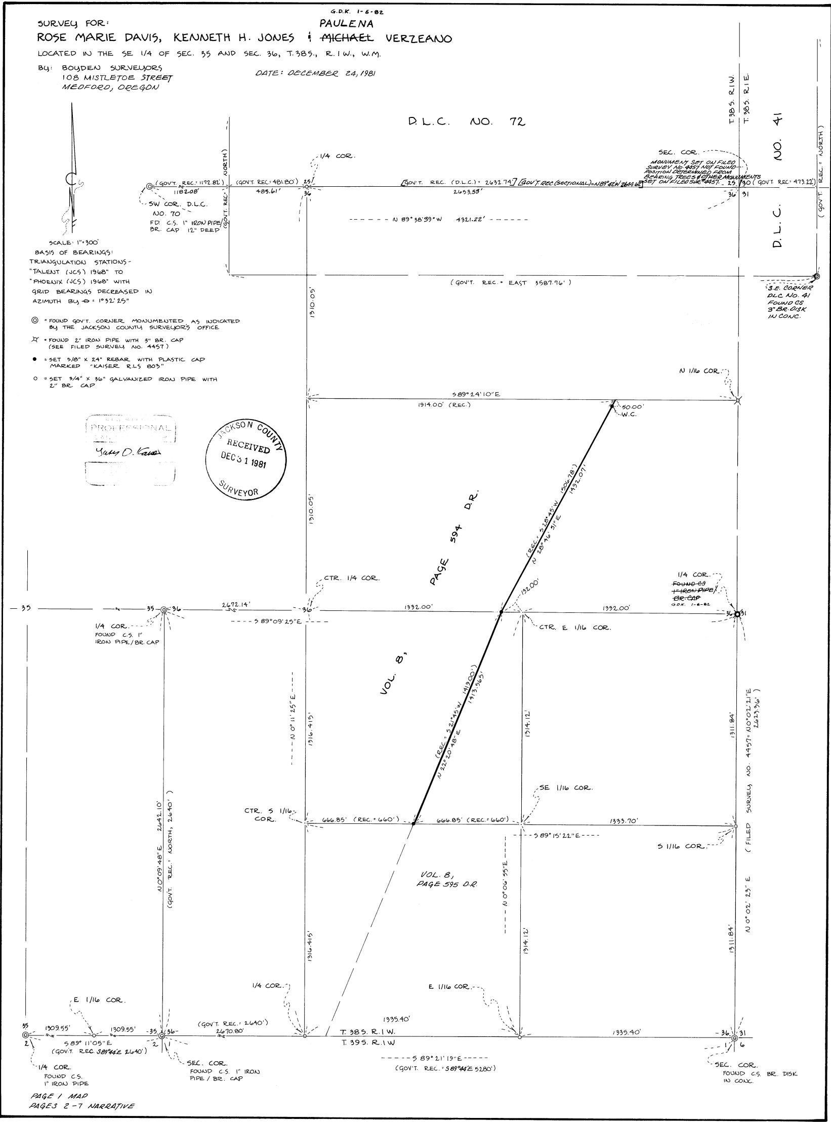
set a 3/4" x 36" galvanized iron pipe 34" in the ground with a 2" bronze cap marked:
