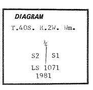
Description of corner evidence found: At corner location, I found a 38-inch diameter pine snag with scribe marks / S visible on open burnt blaze. Using this tree as a reference, I then re-establish the original corner at record distance and bearing. From this corner location I also found a cluster of madrone trees at the record location; however, I was unable to locate the original tree.
