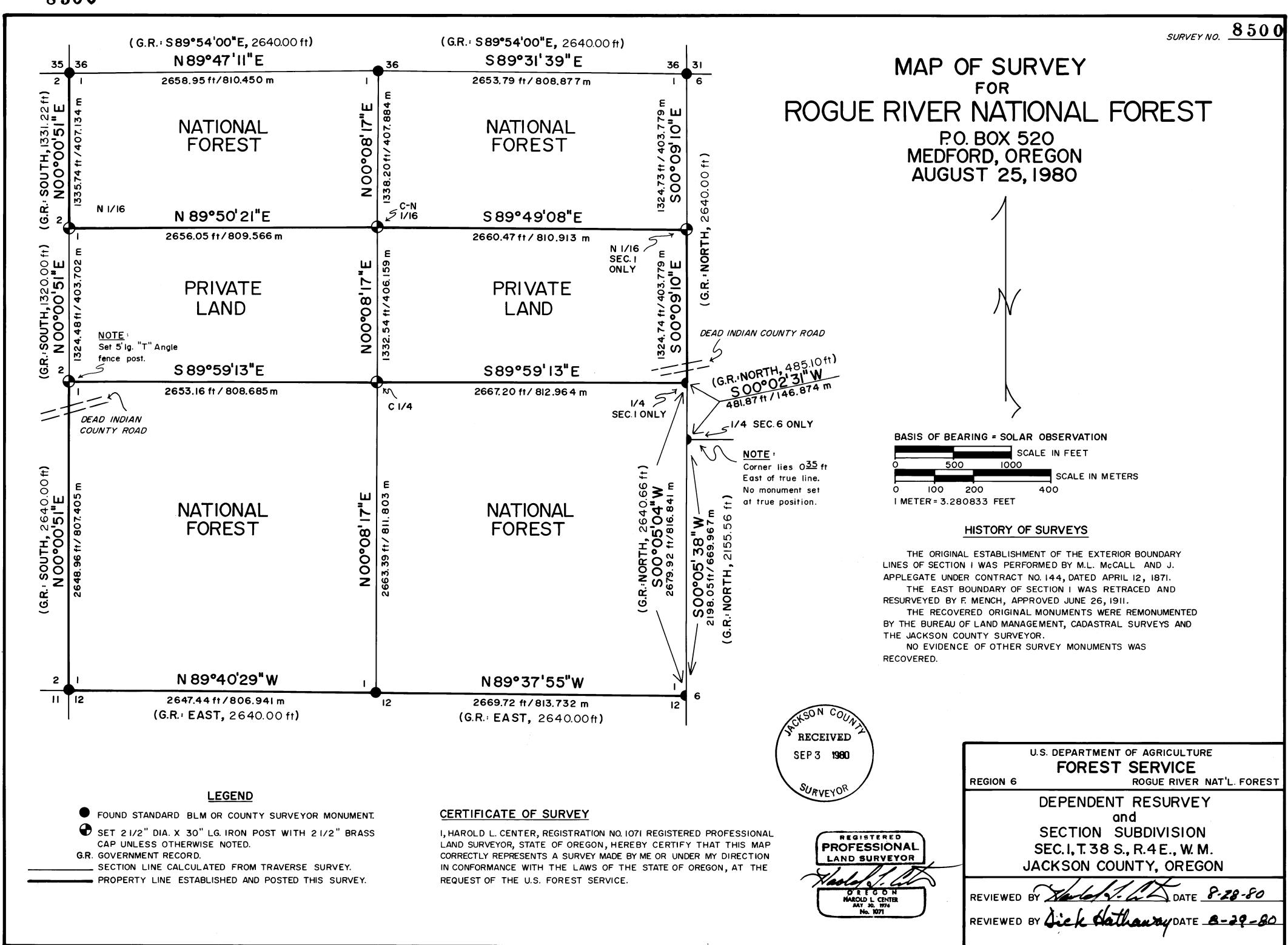
At the corner point I set a  $2\frac{1}{2}$ -inch diameter galvanized iron post with a  $2\frac{1}{2}$ -inch diameter brass cap marked:
