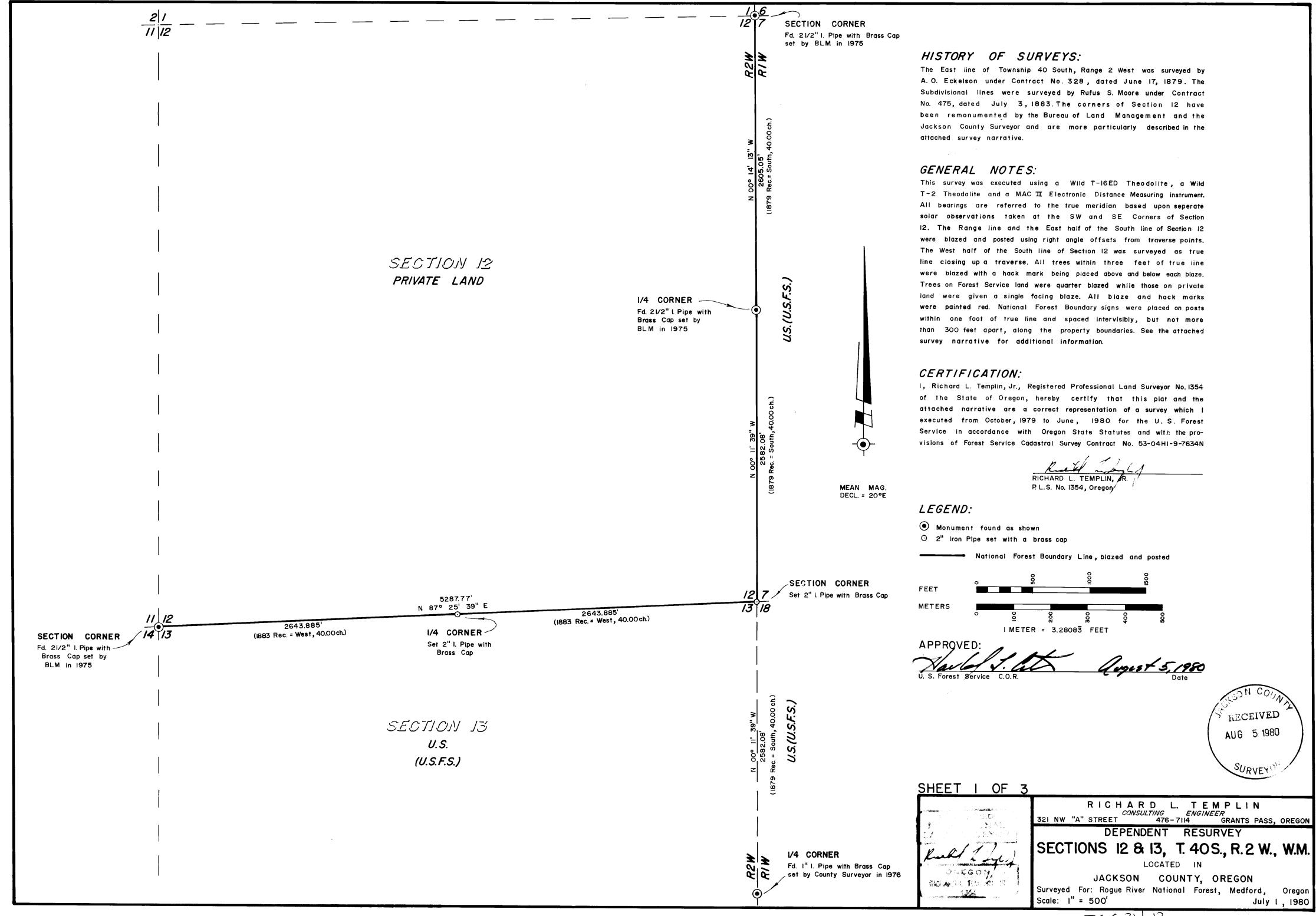
and MAC II E.D.M. The bearings are referred to the true meridian based upon several seperate solar observations made at different locations, as stated on the accompanying plats.
