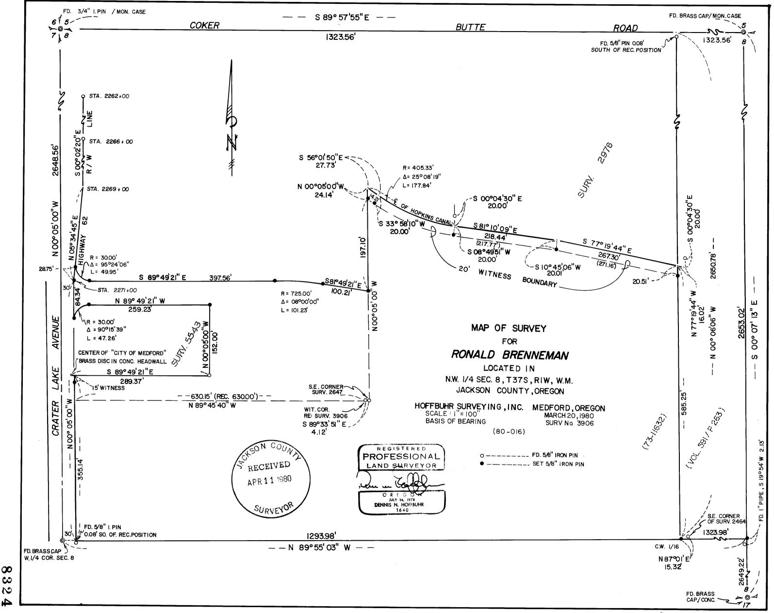
recreated by comparing the calculated distance directly between the found witness monuments with the measured distance (501.58 feet vs. 501.44 feet), and the corresponding proportionate distances were used along the canal.
