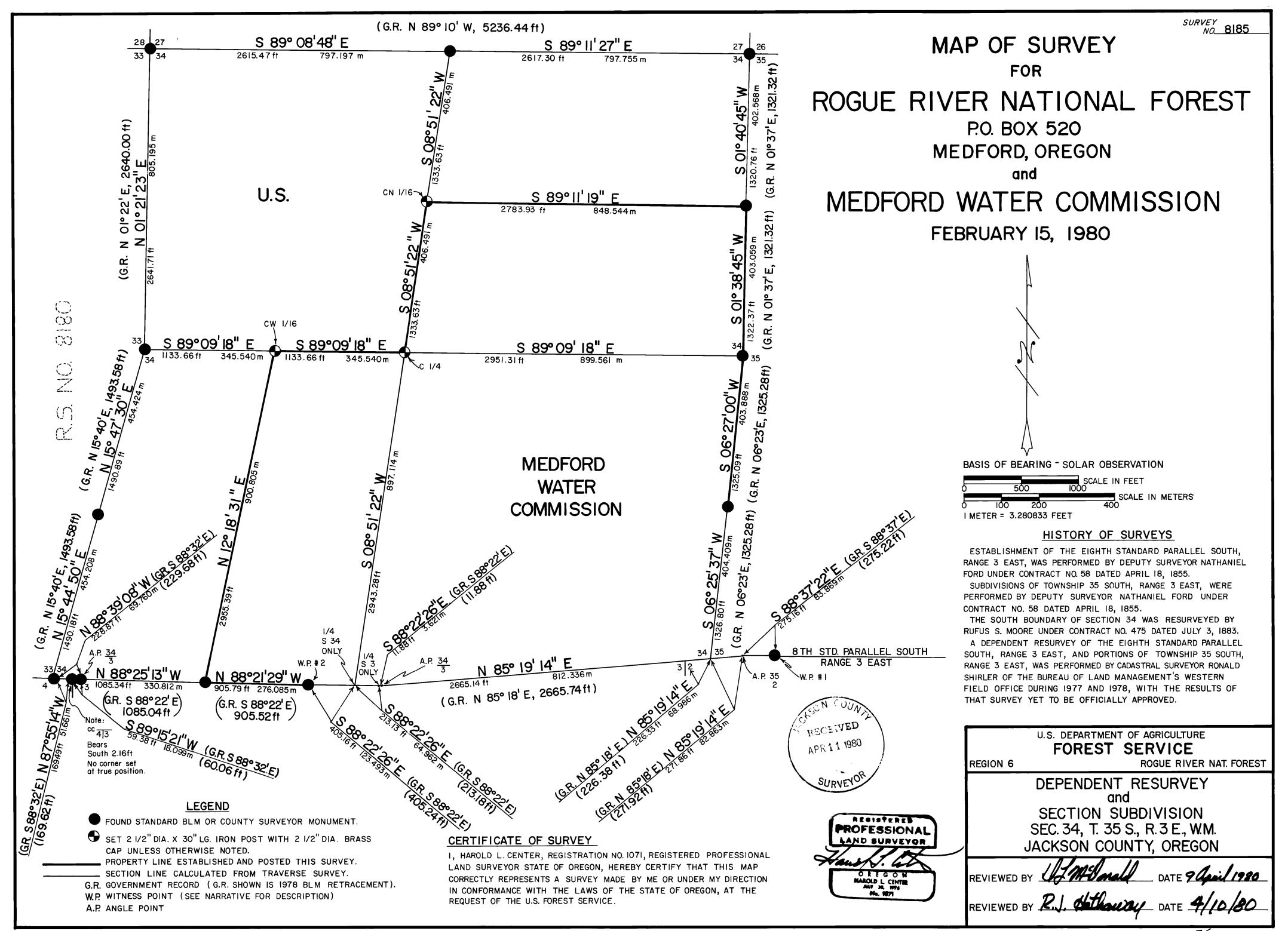
At the corner point I set a  $2\frac{1}{2}$ -inch diameter 30-inch long galvanized iron post with  $2\frac{1}{2}$ -inch diameter brass cap marked:
