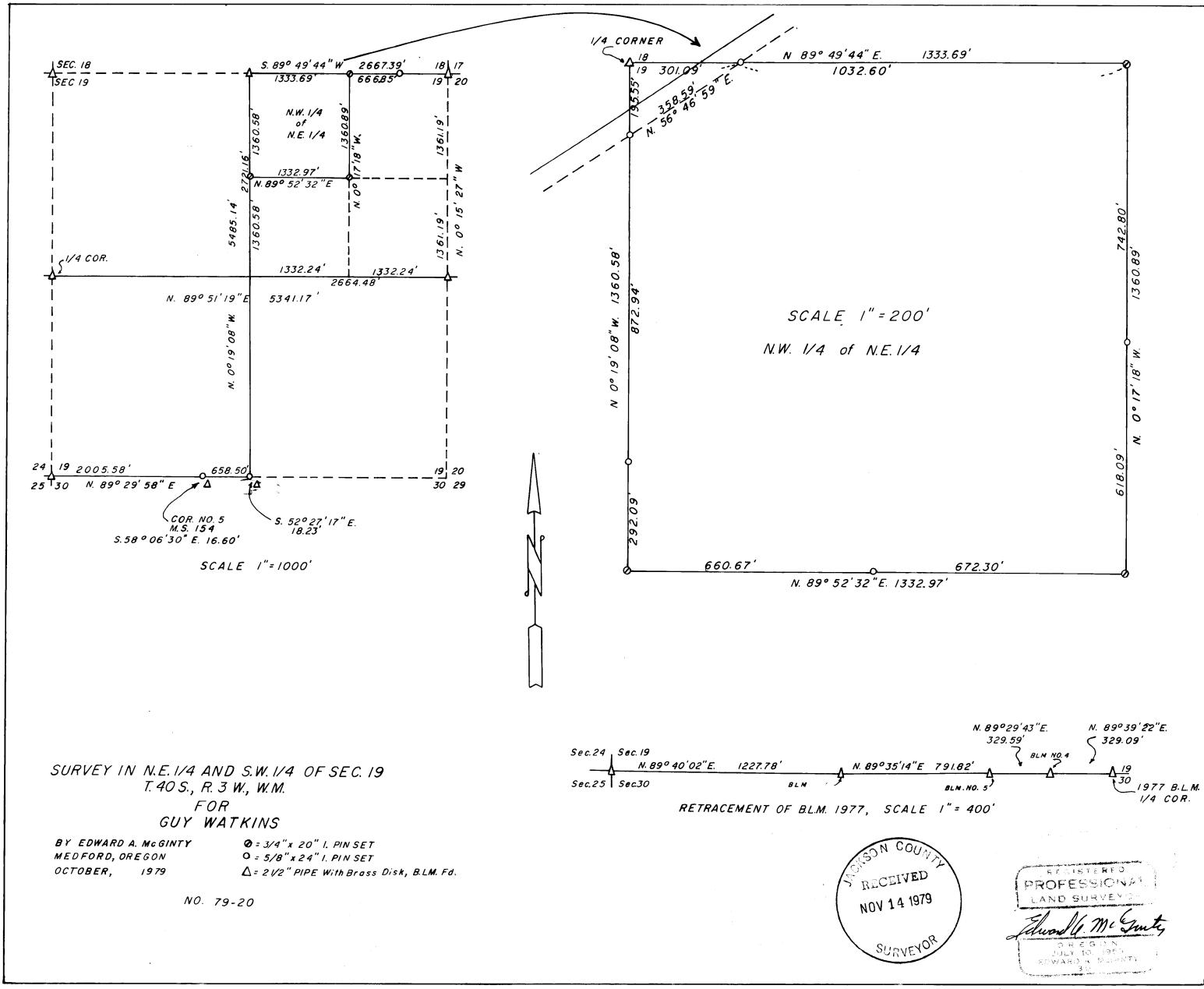
CORNER NO. 5, MINERAL SURVEY NO. 154, found a standard Jackson County, brass disc on a l inch pipe, set flush with the surface, set in 1979, from which
