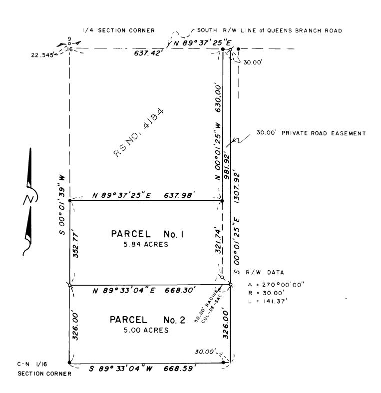
HOFFBUHR SURVEYING, INC. MEDFORD, OREGON SCALE 1"= 200' MARCH 5 ,1979 BASIS OF BEARING R/S No. 4184 2 SET 5/8" x 24" IRUN PIN ●= FD. 5/8" IRON PIN
