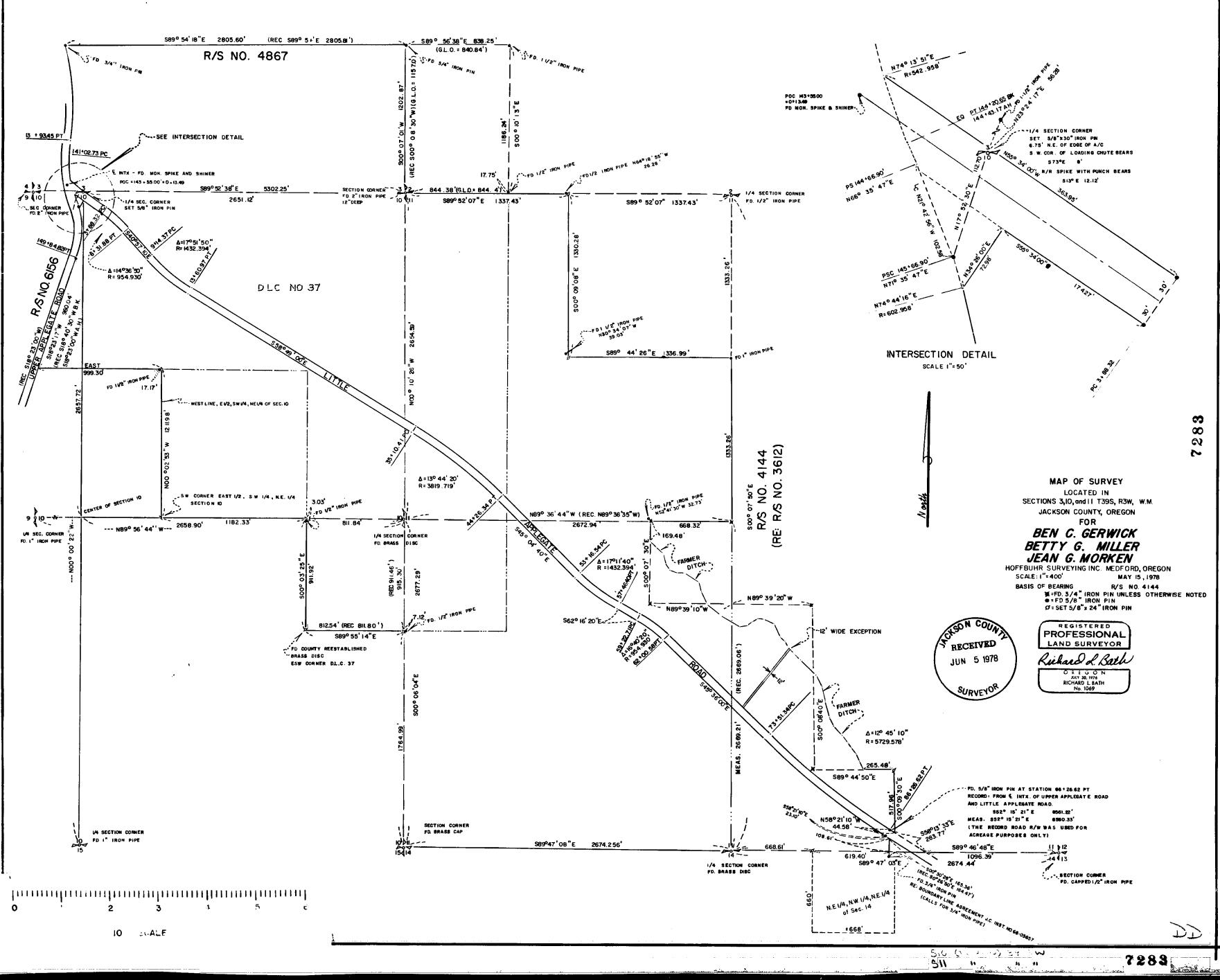
identical by coincidence only. A discrepancy of -0.89 feet in a record distance of 8561.22 feet was adjusted in the tangent distances between the curves along the rights of way. Since there was no attempt to verify all of the monuments along the road right of way, these adjusted right of way distances are to be used for description and acreage purposes only.
