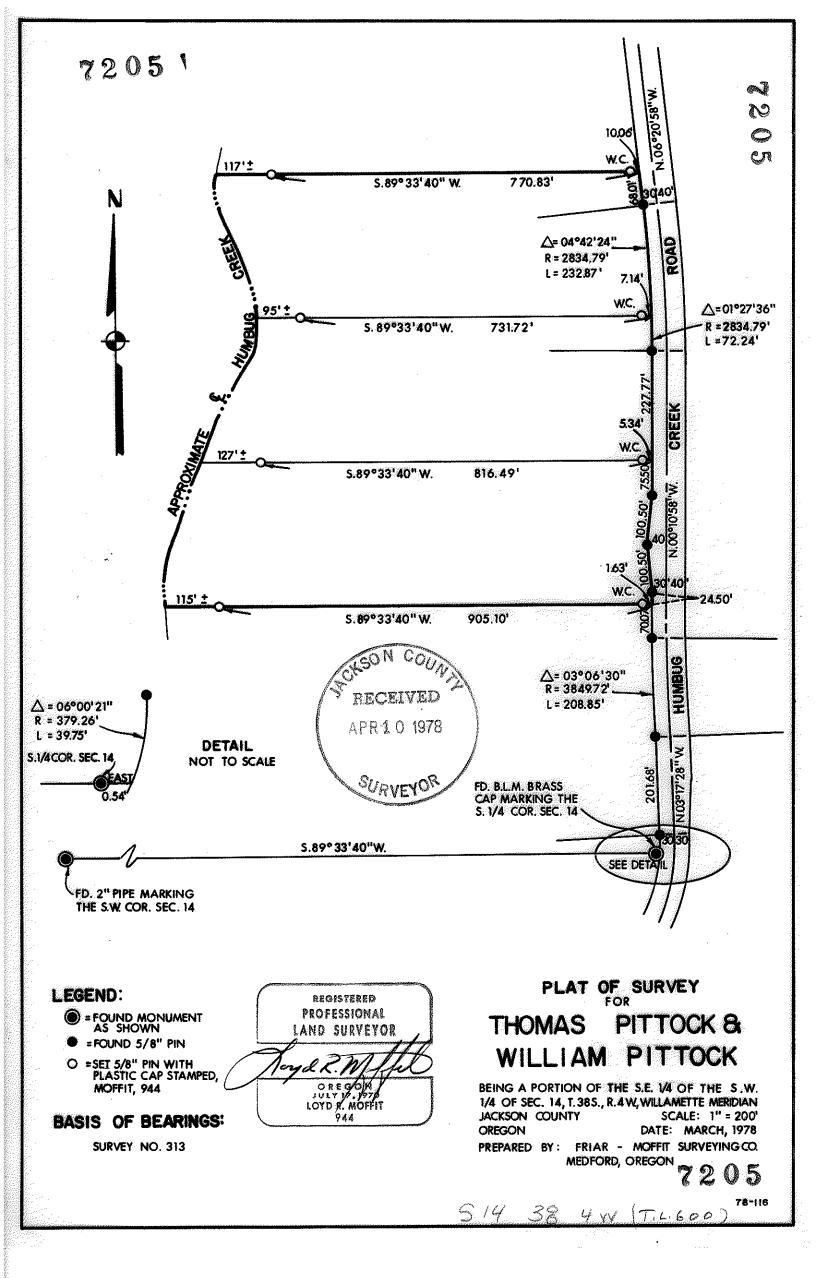
TIES WERE MADE TO PINS SET BY THE COUNTY ROAD DEPARTMENT ON THE WESTERLY RIGHT-OF-WAY LINE OF HUMBUG CREEK ROAD. SAID PINS VARY BY APPROXIMATELY ONE-HALF (1/2) FOOT FROM THE INTENDED LOCATION SHOWN ON SURVEY NO. 5209. COUNTY ROAD DATA AS SHOWN ON SAID SURVEY WAS HELD AND NO ATTEMPT WAS MADE TO ADJUST SAID COUNTY PINS TO THEIR CORRECT LOCATION IN THE FIELD.
