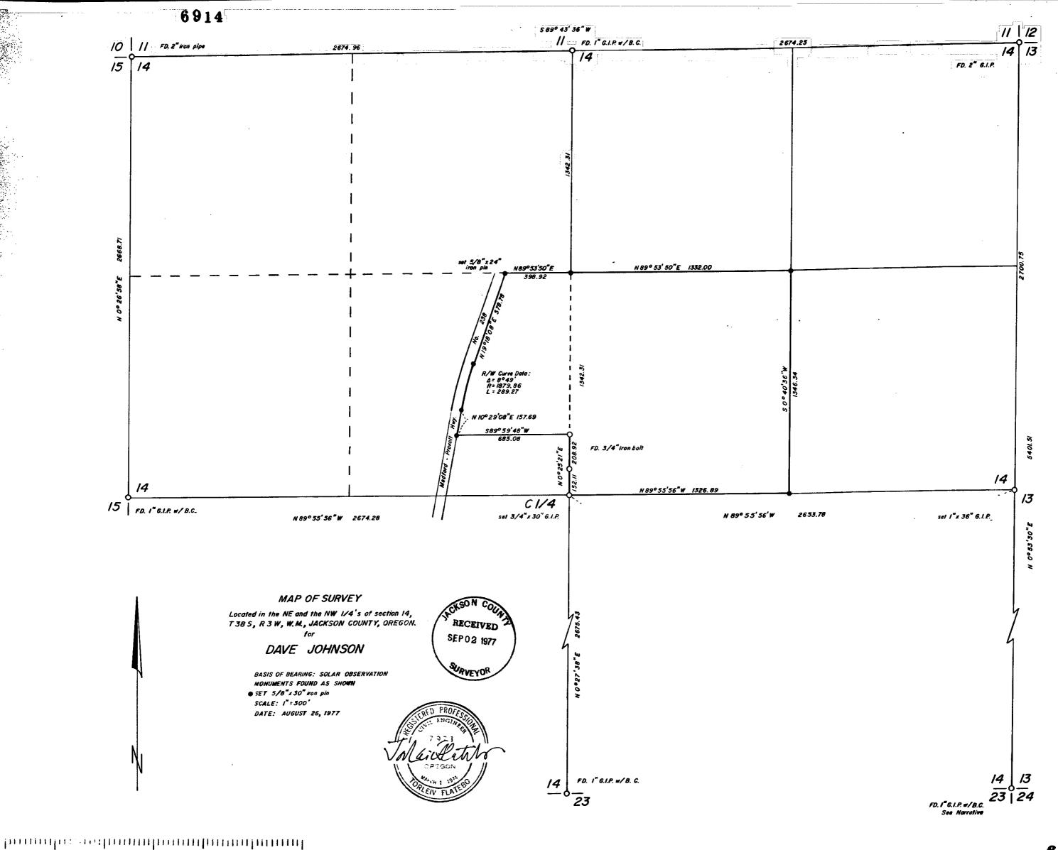
An intensive search was made for the a corner common to sections 14 and 13, yielding no evidence. The corner was set on a proportion basis between adjacent section corners. The proportionate position fit the topog call to the north within a half chain.
