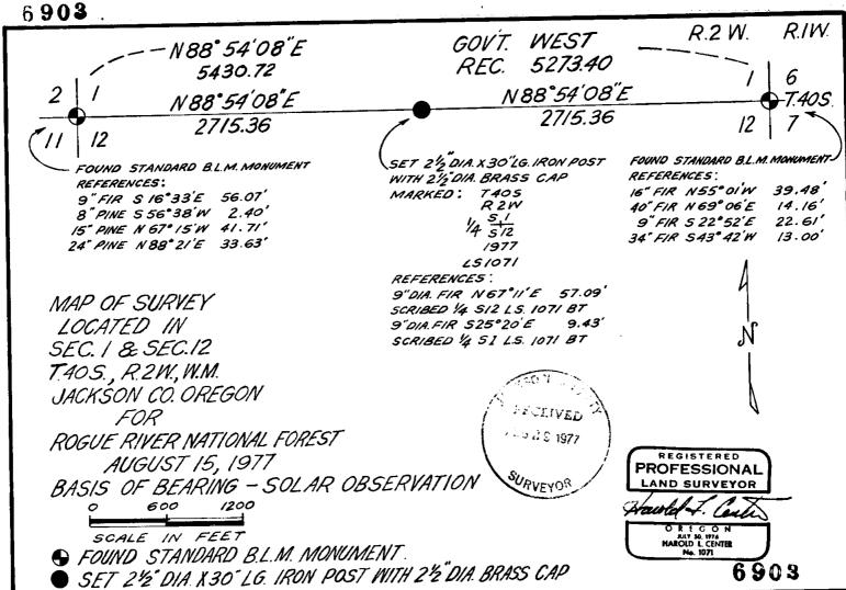
The corner common to Sections 1, 2, 11 and 12, Township 40 South, Range 2 West, at the corner point, I found a 2½ inch diameter galvanized iron pipe with 3 inch brass cap marked:
