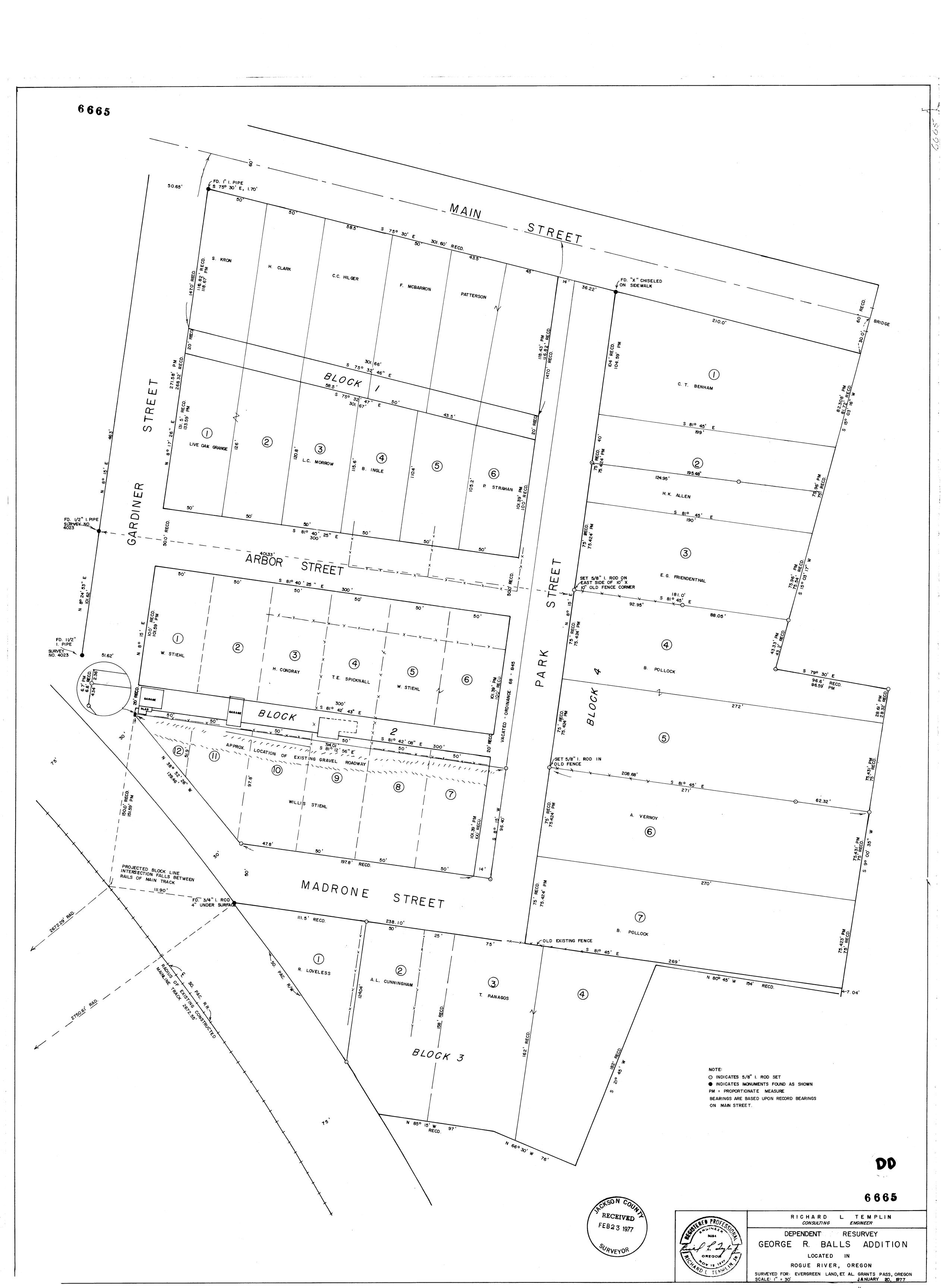
However, Improvements in Block 1 and Block 2 have apparently been made using a distance of 147 feet as the north and south width of the "Smithline Block" resulting in streets and fences being constructed approximately 38 feet too far south. These lines of occupancy are approximately shown on the plat and include structures occupying the alley in Block 2.
