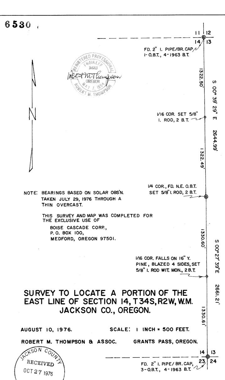
Survey to Locate a Portion of the East Line of Section I4, T34S R2W, W.M., Jackson County, Oregon
