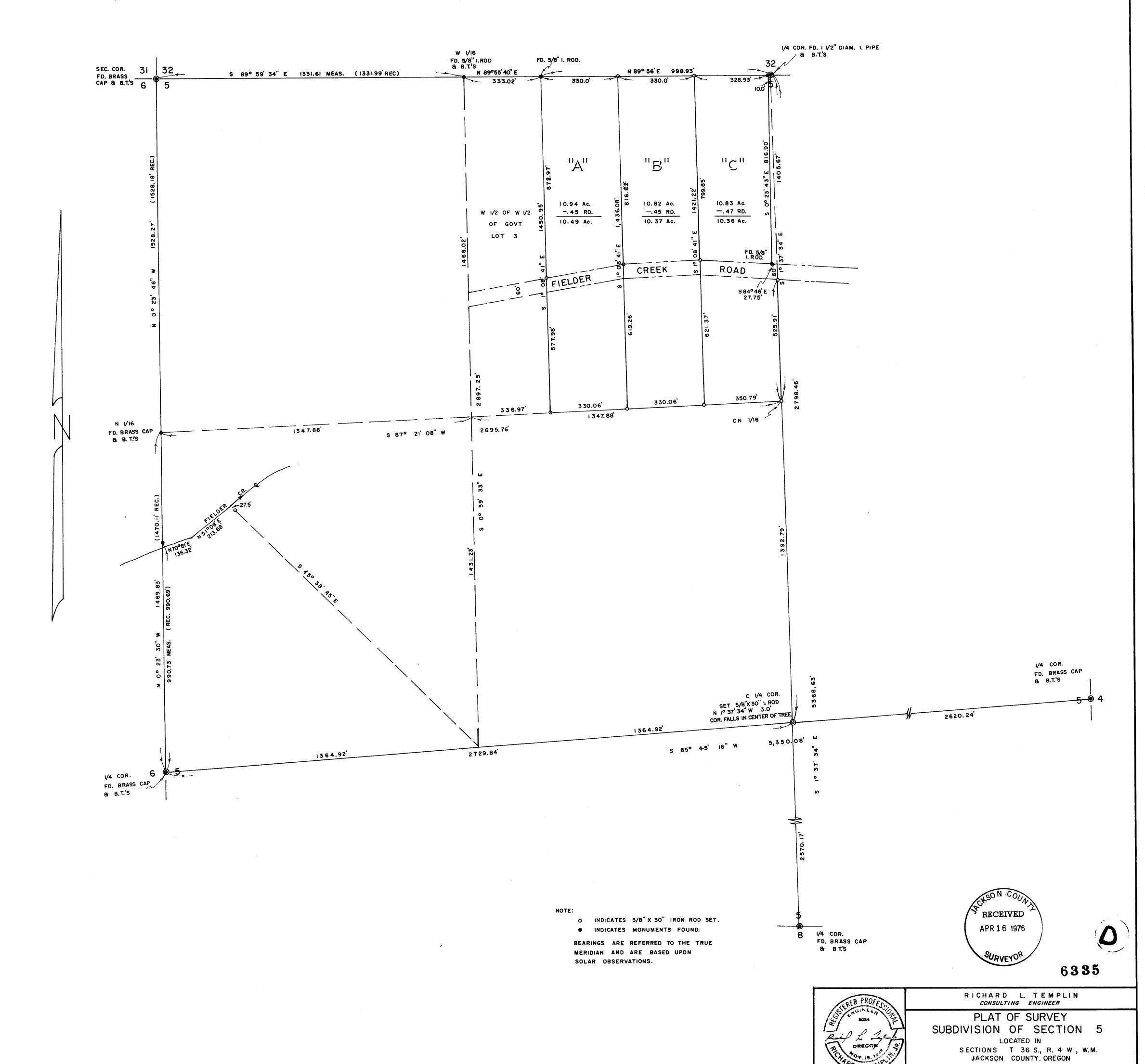
Surveyed For: Mrs. E. I. Green Scale: 1" = 200' Grants Pass, Ore. Apr.il 15, 1976. Thence North 80°23'38" West, 1,469.83 feet to the N 1/16 cor. on the West line which is monumented with a 1976 B. L. M. brass cap and bearing trees;
