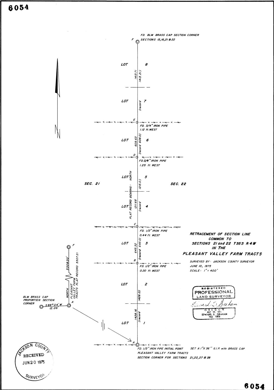
F. Found B.L.M. brass cap section corner common to Sections 15, 16, 21, and 22, T35S, R4W, which was set from a 1953 County Surveyor re-establishment in 1961.
