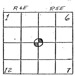
ORIGINAL DESCRIPTION: Set a sandstone 14" x 12" x 10" from which: A White Oak, 12" in diameter, bears N42°W, 90 Lks. distance A White Oak, 14" in diameter, bears N61°E, 200 Lks. distance A White Oak, 24" in diameter, bears S49°W, 148 Lks. distance
