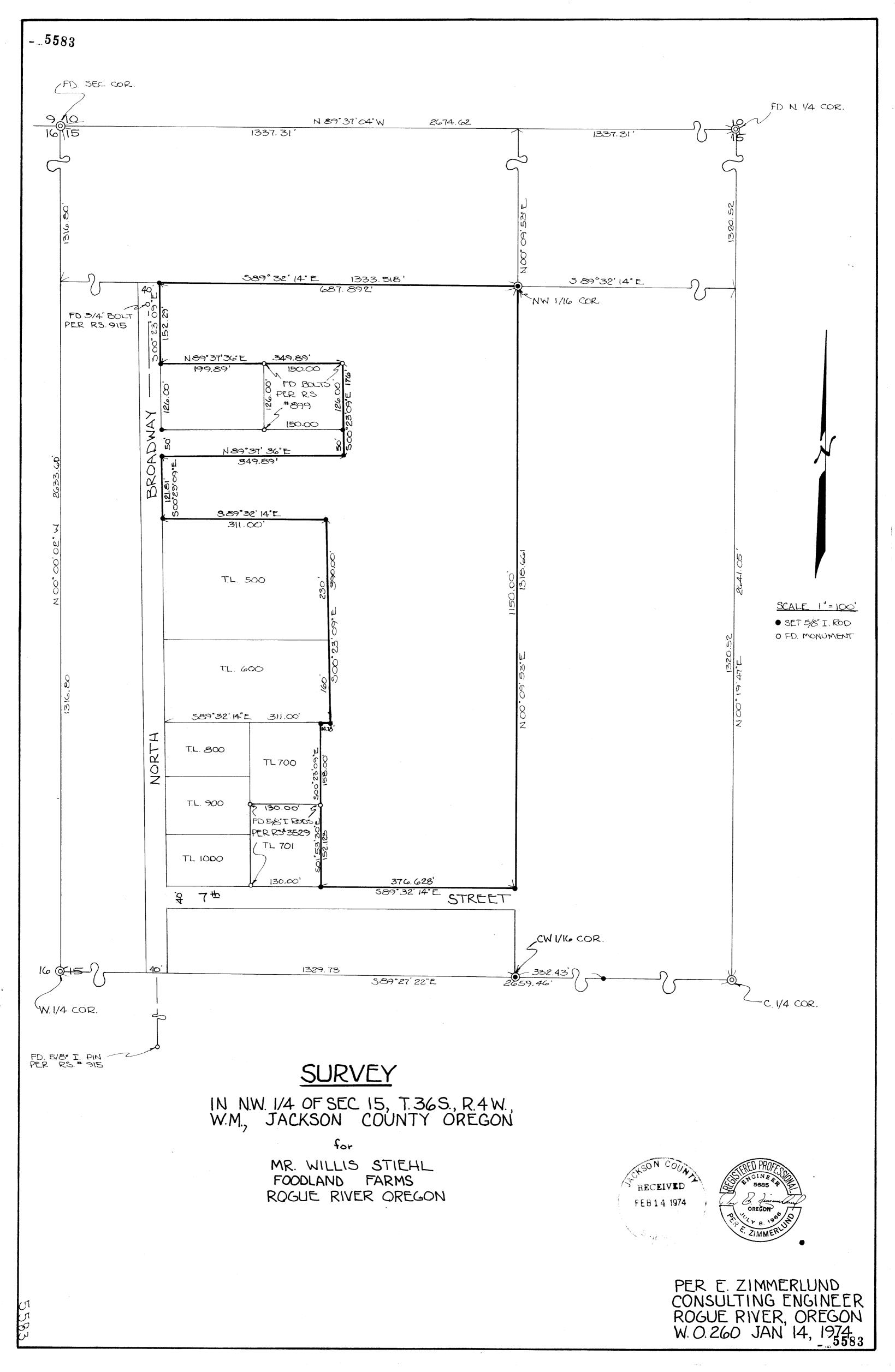
S 01°53'30" E 152,123 feet to the North right of way line of 7th Street, at which point I set a 5/8" x 30" iron rod; thence I run S 89°32'14" E along the North right of way line of 7th Street 376.63 feet to a previously set 5/8" x 30" iron rod.
