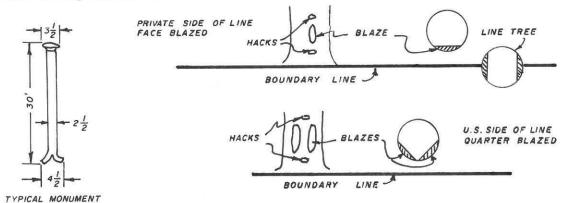
În areas of sparse timber growth some trees were marked in excess of 7 feet from the true line. All blazes and hack marks extend into the live wood tissues of the tree. Boundary signs were posted on trees at intervals of 660 feet or less along the lines.
