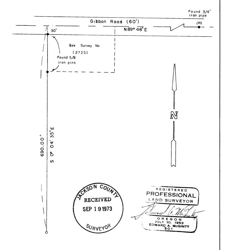
Survey in DLC 55 & SE 1/4 Sec 26, T36S, R2W, W.M.
