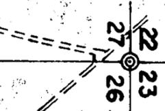
SEC. COR., FND. 2 1/2" I. PIPE W/B.L.M. BR. CAP, DISPLACED, S 51° 33' E 1.36 LKS. FROM TRUE COR. AS MEAS. FROM O.B.T.'S & NEW B.T.'S. FND. PER B.L.M. 1958 RENEWAL.
