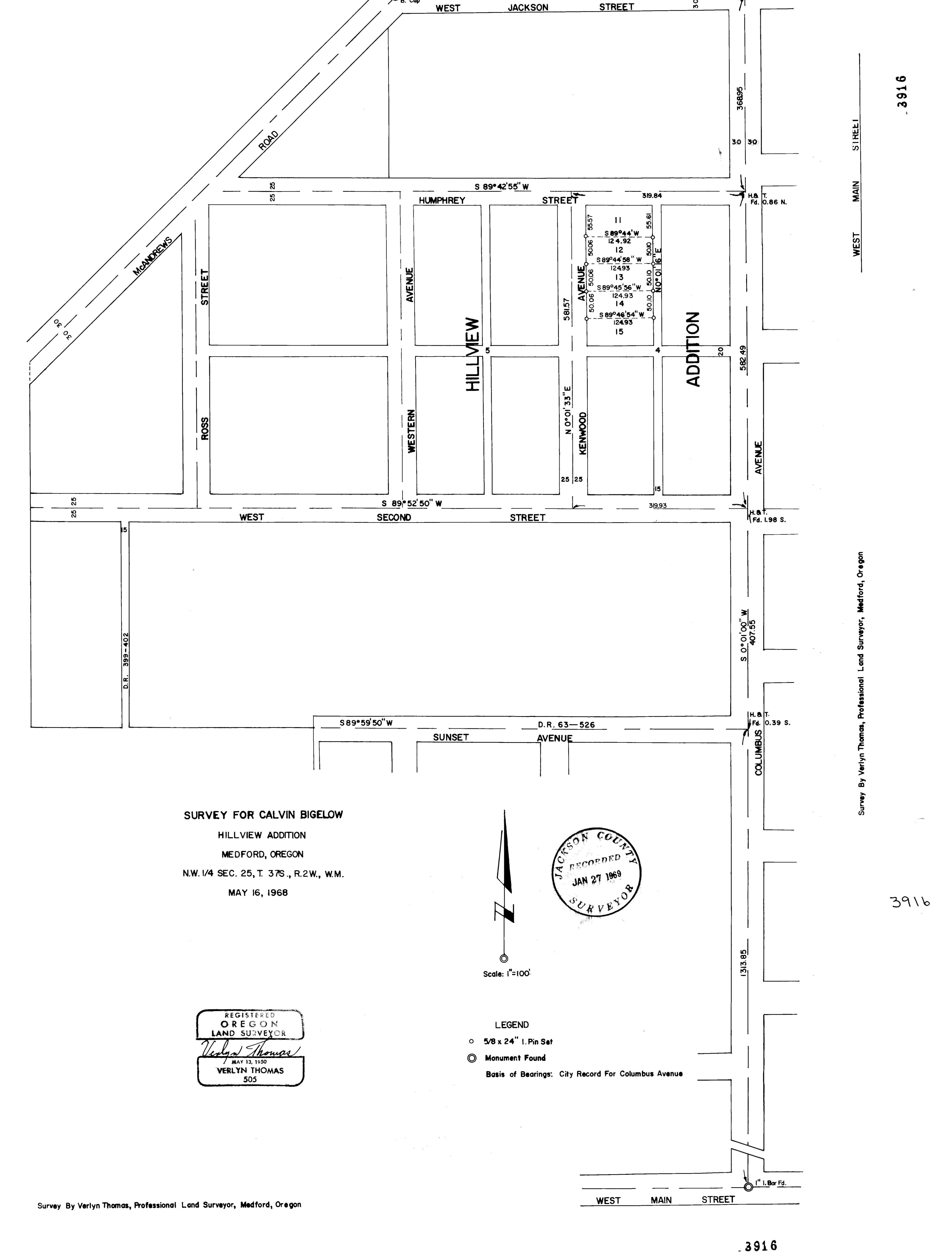
Based upon these conclusions, a survey was conducted tieing in original monuments shown on the Plats of WESTERN ADDITION and RICHMOND ADDITION, the 1 Corner between Sections 26 and 25, the 1 Corner between Sections 24 and 25, and numerous other monuments called for in old deed descriptions.
