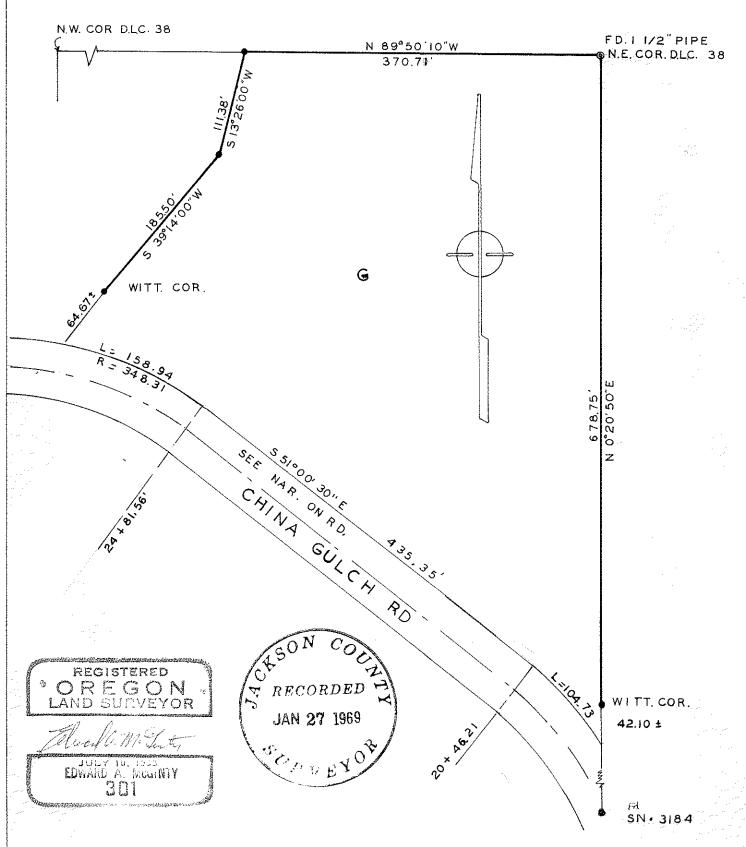
SURVEY IN N.E. 1/4 SEC. 28 T.38S. R.3 W. W.M.
