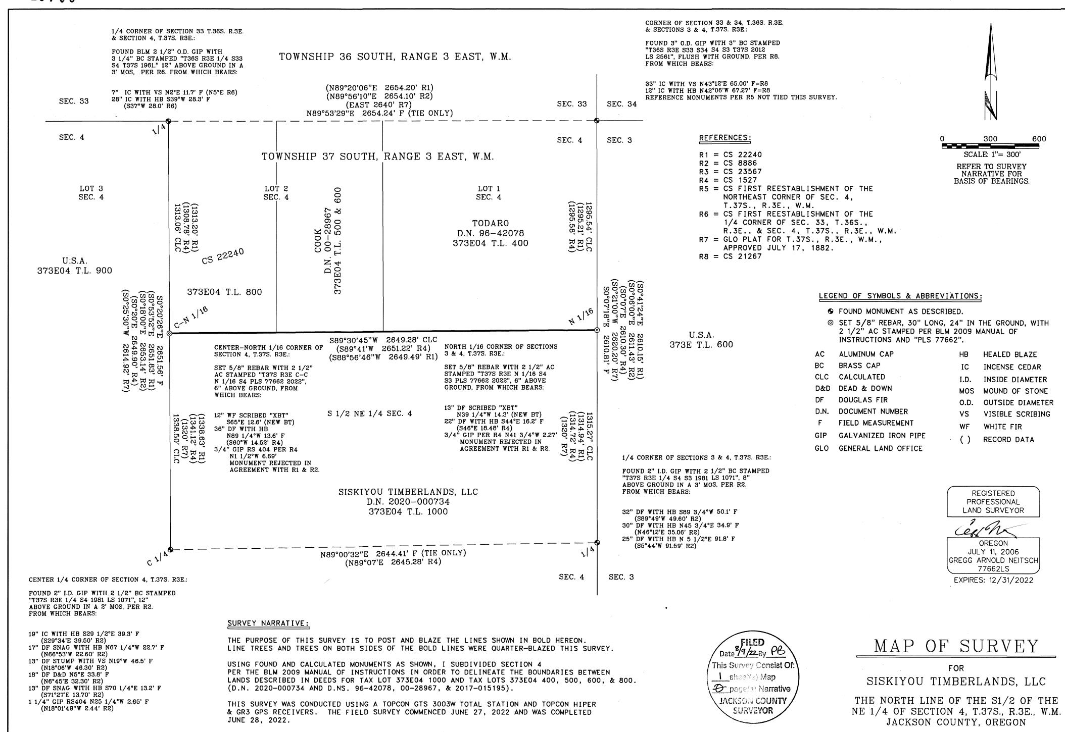
THE BASIS OF BEARINGS FOR THIS SURVEY IS GEODET!C (NAD83), AT THE SOUTHWEST CORNER
