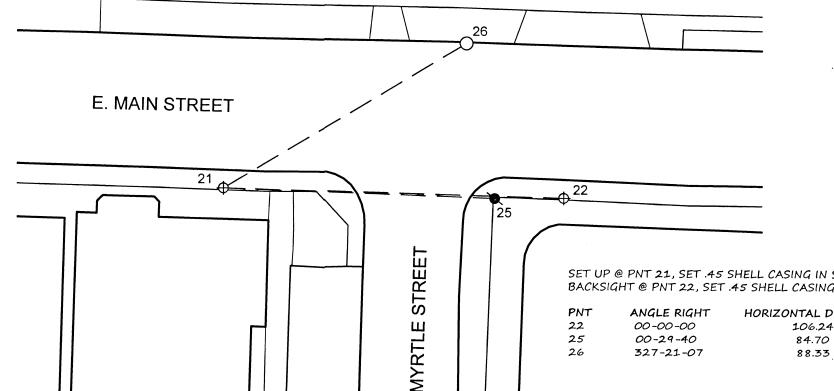
SET UP @ PNT 21, SET .45 SHELL CASING IN SIDEWALK BACKSIGHT @ PNT 22, SET .45 SHELL CASING IN SIDEWALK
