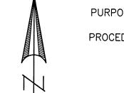
BASIS OF BEARINGS G.P.S. NAD 83 [2011] - PROJECTED ON TO GRID BEARING PER OREGON COORDINATE REFERENCE SYSTEM
