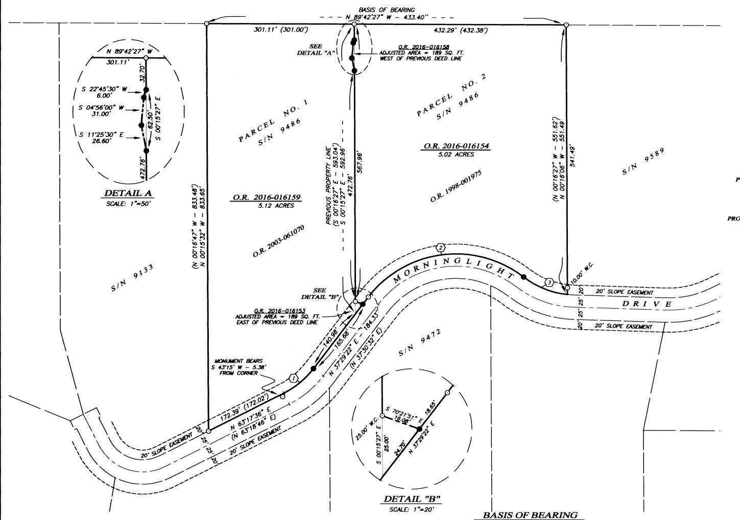
THE BASIS OF BEARING FOR THIS SURVEY IS THE EAST-WEST CENTERLINE OF SECTION 23, LOCATED WITHIN TOWNSHIP 39 SOUTH, RANGE 1 EAST OF THE WILLAMETTE MERIDIAN, HAVING A RECORD PLAT BEARING OF NORTH 89°42'27" WEST, AS REFERENCED ON SURVEY NO. 9486, ON FILE IN THE OFFICE OF THE JACKSON COUNTY SURVEYOR.
