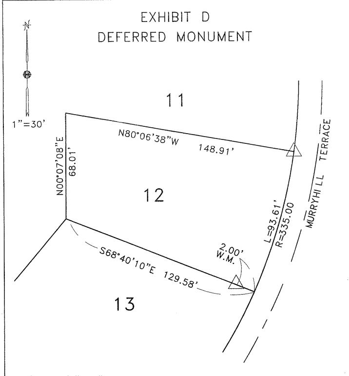
$\triangle$  = 5/8"X24" REBAR WITH PLASTIC CAP STAMPED "HOFFBUHR & ASSOC, INC"
