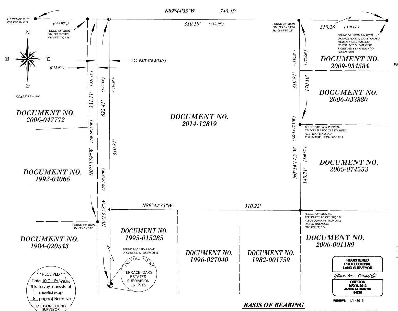
THE BASIS OF BEARING FOR THIS SURVEY IS THE FOUND NORTHWEST IRON PIN OF DOCUMENT NO. 2006-047772 AS DETERMINED BY SURVEY NUMBER 4521 AND THE FOUND IRON PIN OF THE NORTHEAST CORNER OF LOT 24 OF FAIRVIEW SOUTH CHILDERS EASTERN ADDITION AS DETERMINED ON SURVEY NUMBER 15021, AS RECORDED IN THE OFFICIAL RECORDS OF JACKSON COUNTY, OREGON. IN SECTION 20, TOWNSHIP 37 SOUTH, RANGE 1 WEST OF THE WILLAMETTE MERIDIAN, JACKSON COUNTY, OREGON
