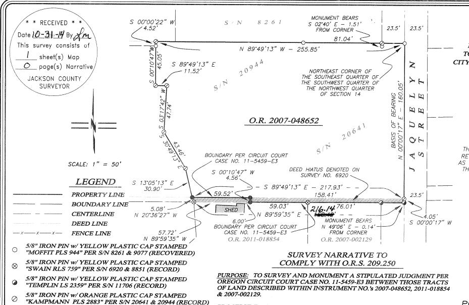
PROCEDURE: UTILIZING AN ELECTRONIC LEICA TCRP 1203 ROBOTIC TOTAL STATION AND RANGING PRISMS, ALONG WITH SURVEY CONTROL PREVIOUSLY ESTABLISHED BY THIS OFFICE DURING THE PERFORMANCE OF SURVEY NO. 20641, I ESTABLISH MONUMENTS ALONG A HIATUS STRIP PREVIOUSLY DESCRIBED IN THE SURVEY NARRATIVE FOR SURVEY NO. 6920 & 20641.
