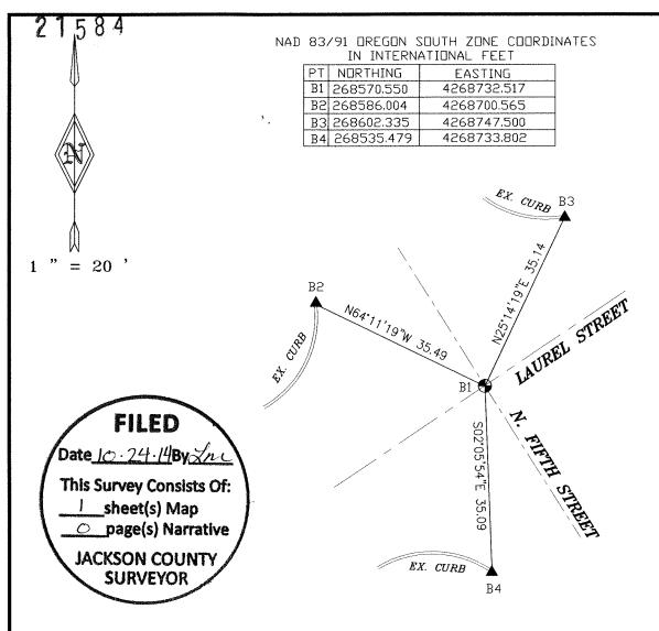
PURPOSE: To replace and reference an existing 2" brass cap monument in a monument well prior to it's destruction by a newly placed sewer line, per 0.R.S 209.150. This monument is located at the centerline intersection of Laurel Street and 5th Street in Central Point, Oregon.
