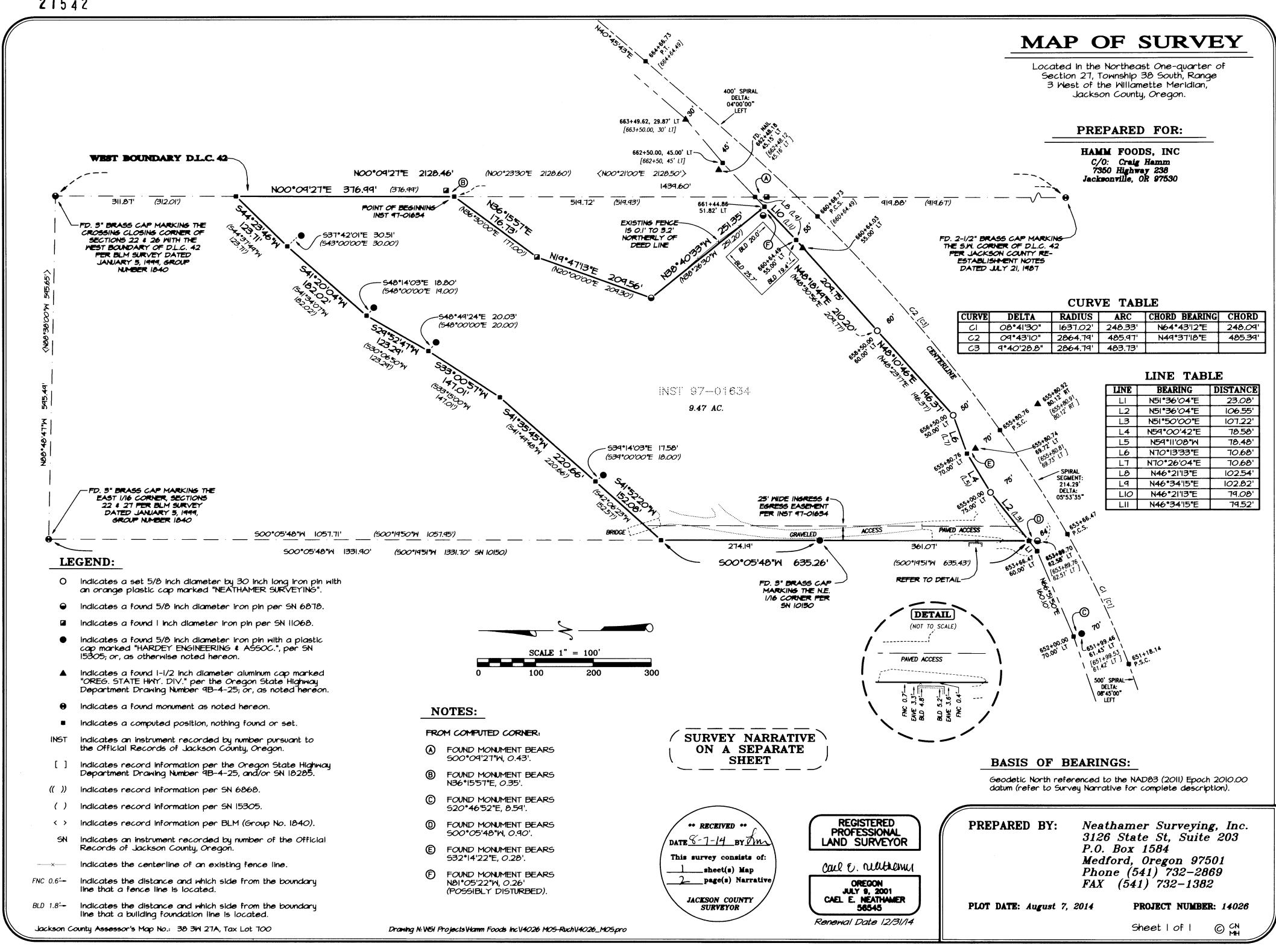
All bearings and distances shown on the accompanying map are projected (grid) values based on the projection definition herein and above. This projection was utilized in order to minimize the difference between projected (grid) distances and horizontal (ground) distances at the topographic surface within the design area of this coordinate system.
