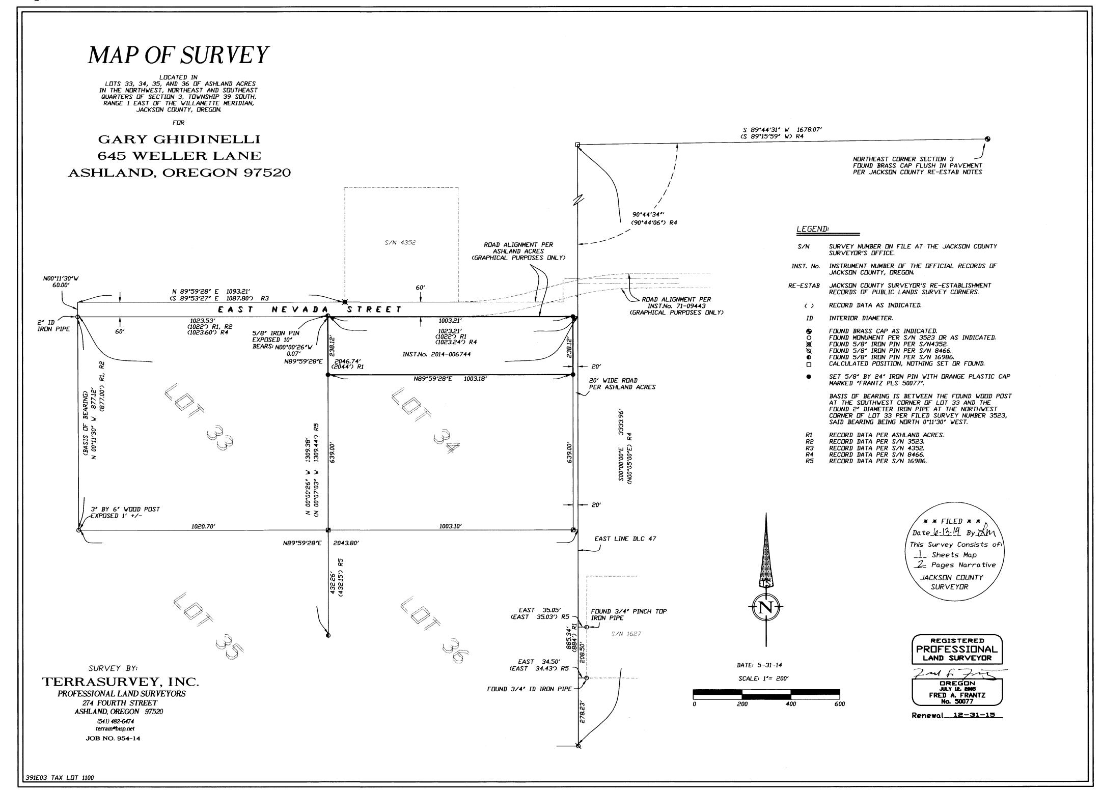
corner and by proportional measurement using record distance calls from government notes along the north line of Section 3 between the north 1/4 corner and the northeast corner of Section 3 and sets the northeast corner of Lot 40 on the Section line.
