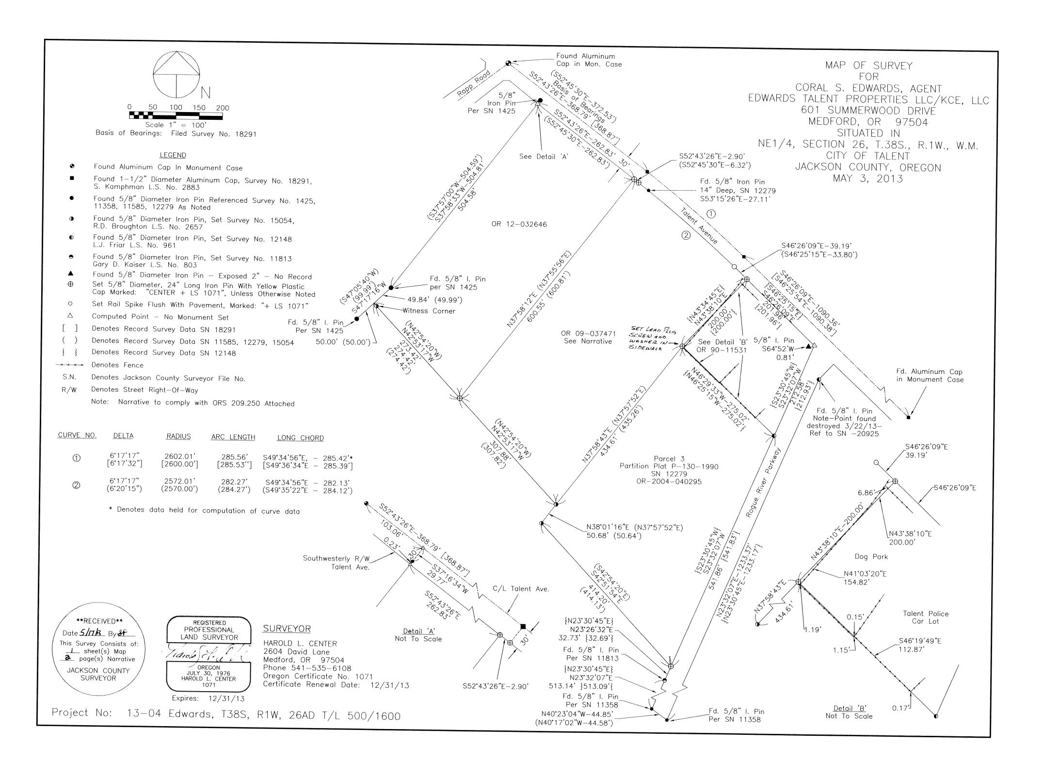
Broughton's survey No. 15054 indicates recovery of the Edwards corner points. Broughton provided no information to indicate he performed sufficient surveying to discover the difference. In addition Broughton's survey map and the description prepared for the property line adjustment deed 96-25687 contain errors in the curve data.
