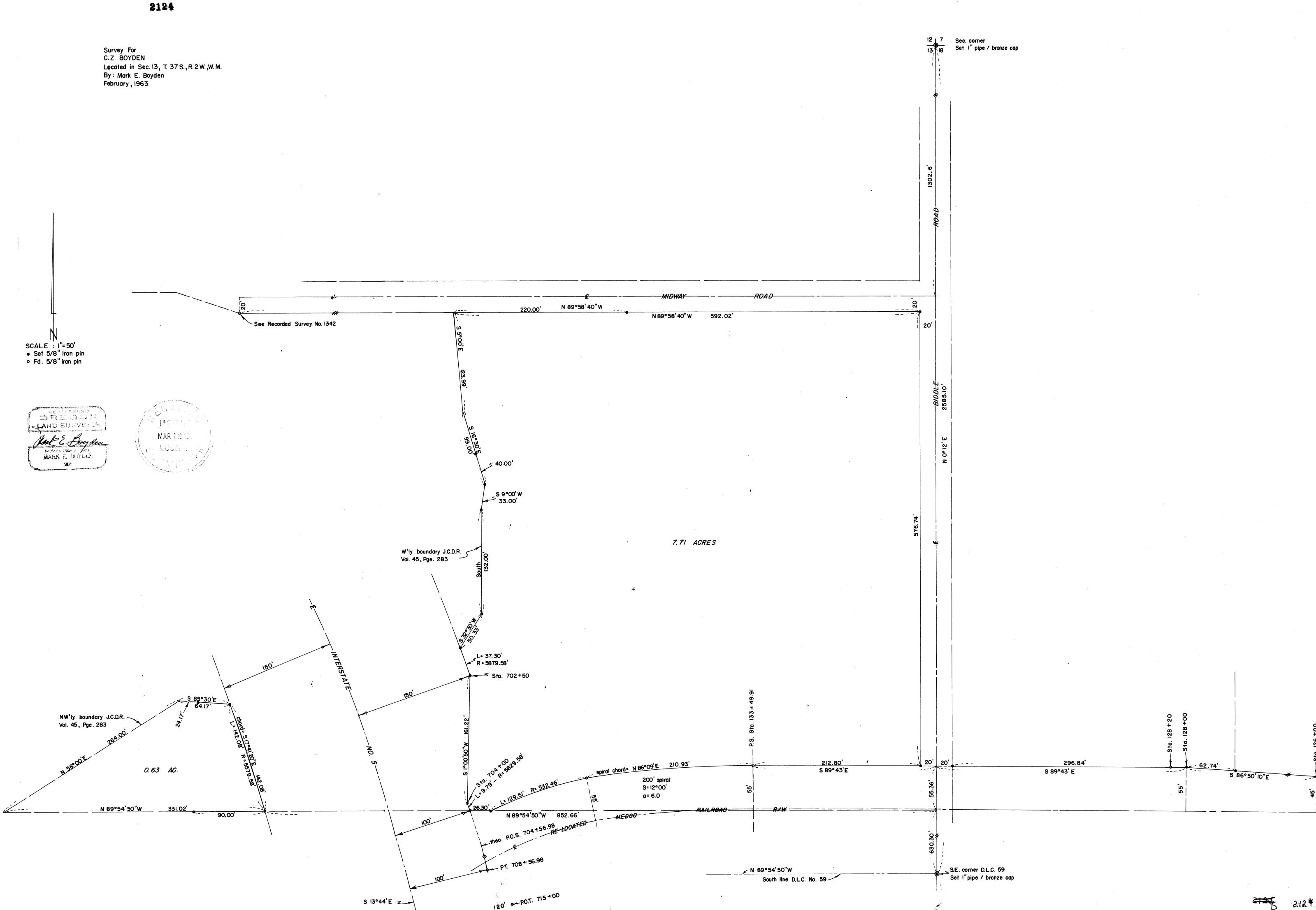
Monumented the parcels with 5/8" iron pins as shown, using for meridian control, the bearing of solar origin determined for the centerline of Biddle Road on Recorded Survey No. 609.
