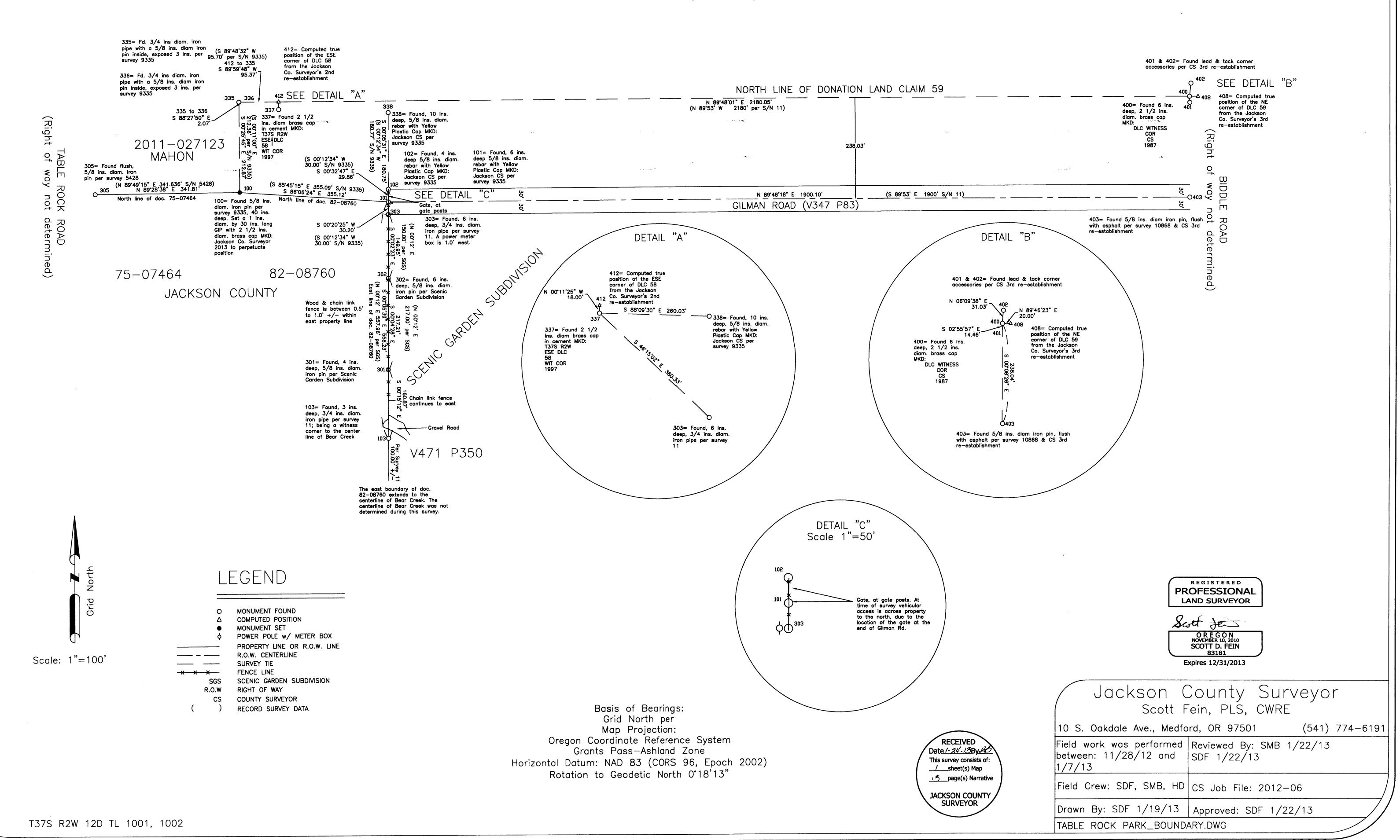
during the course of survey 9335 and was recovered and accepted during the course of this survey (101). The north line of document 82-08760 was determined between points 100 and 101 was marked with temporary wooden hubs.
