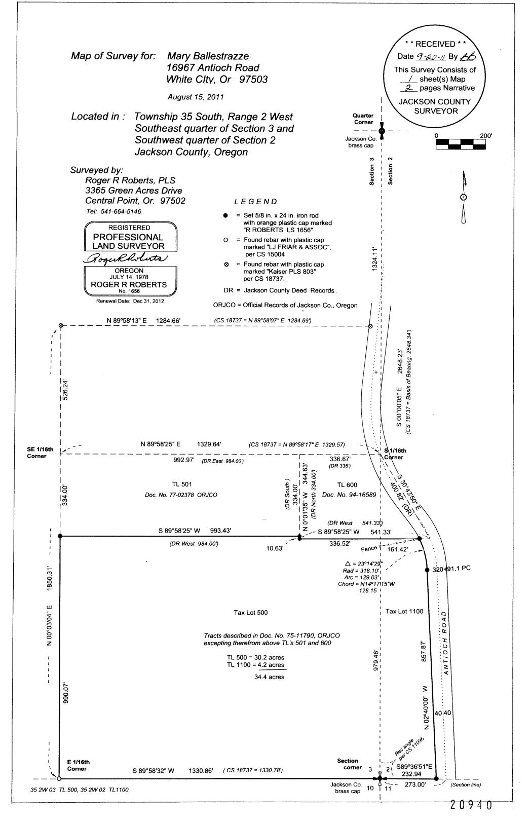
The centerline of the county road 80 ft. right of way was determined from the 1910 road records distance of 273 ft. from the section corner. From this point northerly, the centerline was determined by a best fit of the current asphalt alignment compared with the engineered right of way as indicated in the 1945 County Engineer map of Antioch Road, Sta -0+68.1 to Sta 402+67.4, filed in the Office of County Surveyor as Roll Map 2/3.
