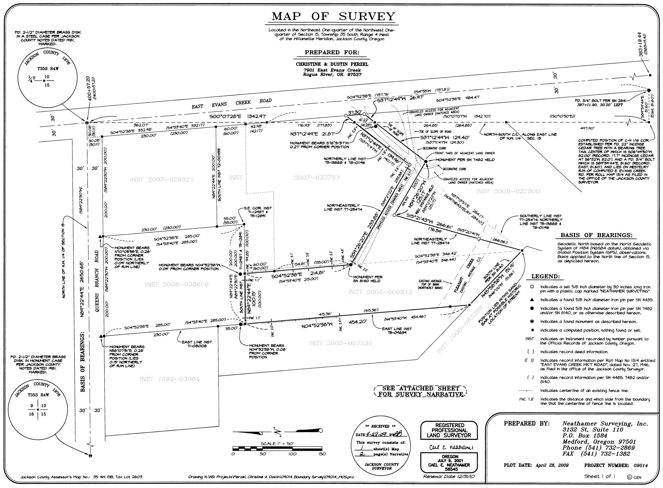
Utilizing said established North-South Center of section line and said North One-quarter corner, rotated and translated Roll Map No. 13/4 onto our local coordinate system and bearing base, establishing the location of East Evans Creek Road right-of-way. It should also be noted that the found 3/4-inch iron bolt, aforementioned reference point per Survey Number 2841, falls within 0.03 of a foot of being on said established right-of-way.
