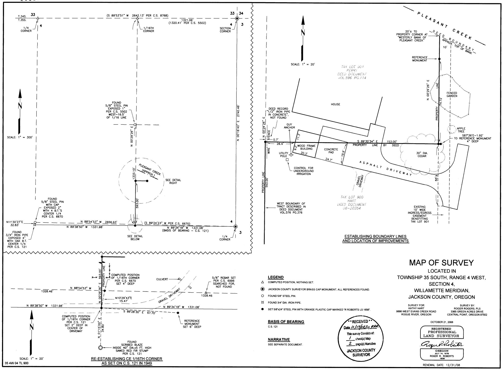
large discrepancy in the location of the C1/4 corner between the two surveys, it was necessary to retrace the Ager survey to determine the accuracy of the CS121 location for the CE 1/16th corner.
