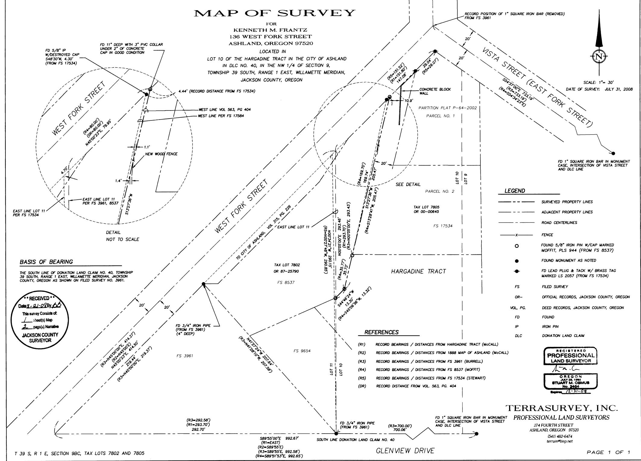
He shows a distance of 598.15 feet along this centerline which compares with a calculated distance of 603.34 feet from the map of the Hargadine Tract.
