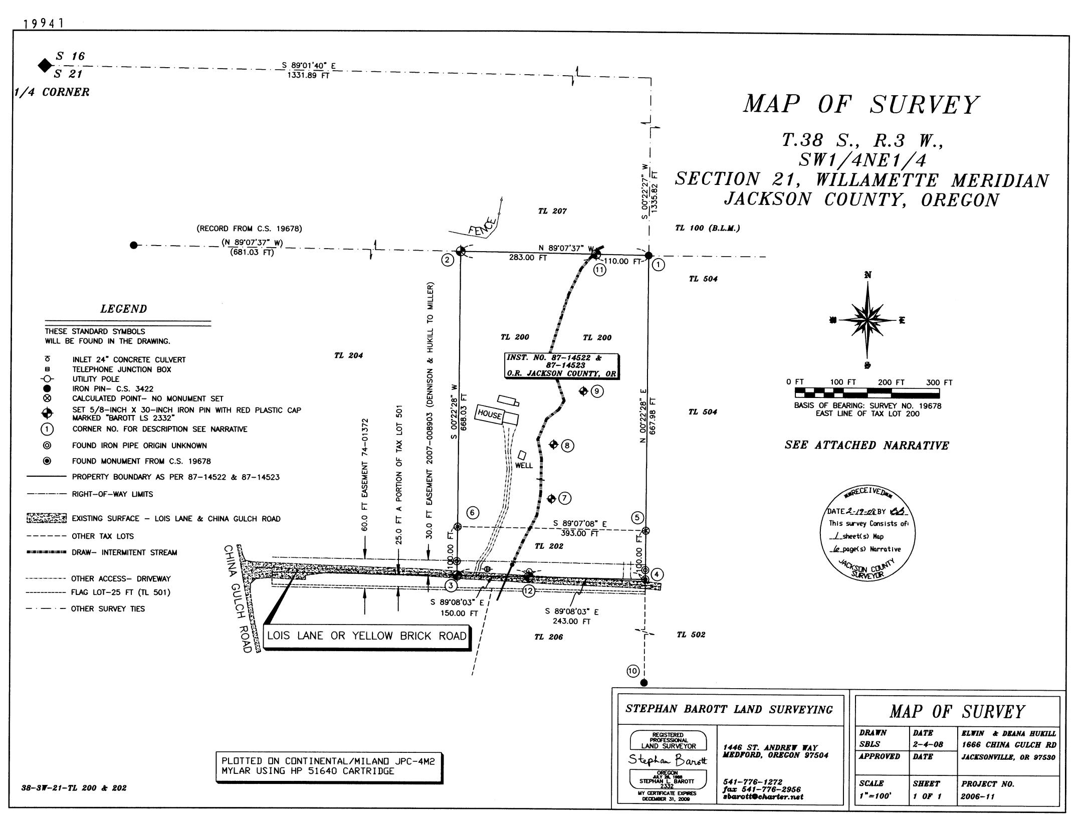
I set a 5/8-inch diameter X 30-inch iron pin, with a red plastic cap marked "BAROTT LS 2332" on the interior of my client's parcel, and East of the draw, North 73°30'14" East, 204.17 feet distance. (Refer to corner 7).
