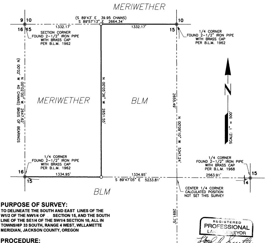
A SERIES OF CLOSED TRAVERSES WERE COMPLETED TYING TO CORNERS AS NOTED UTILIZING A TOTAL STATION AND GPS. THE CENTER 1/16 POSITION WAS CALCULATED AND 1/16 CORNERS WERE SET AS NOTED. TRUE LINE WAS BLAZED AND POSTED AS SHOWN IN **ACCORDANCE TO THE 1973 MANUAL OF INSTRUCTIONS** FOR THE SURVEY OF PUBLIC LANDS OF THE UNITED STATES.
