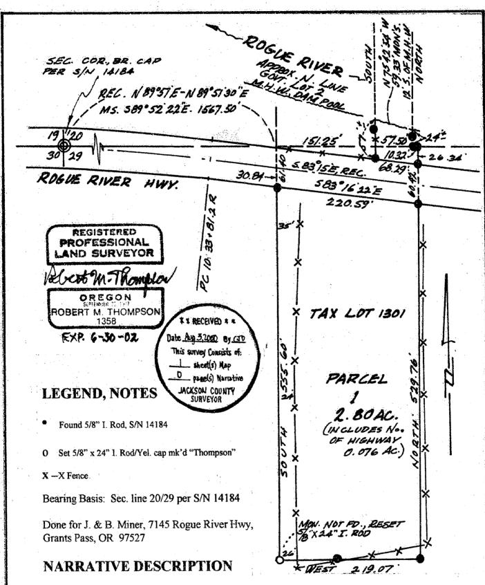
The purpose of this survey was to find all the previously set corners of Parcel 1 of Partition Plat No. P-91-1994, mark the boundaries, and re-set any missing corners. A closed traverse was run around said boundaries, which were then marked up in their true positions, using red painted tree blazes, red flagging, and "glo-top" stakes. The missing Southwest parcel corner was re-set as stated above.
