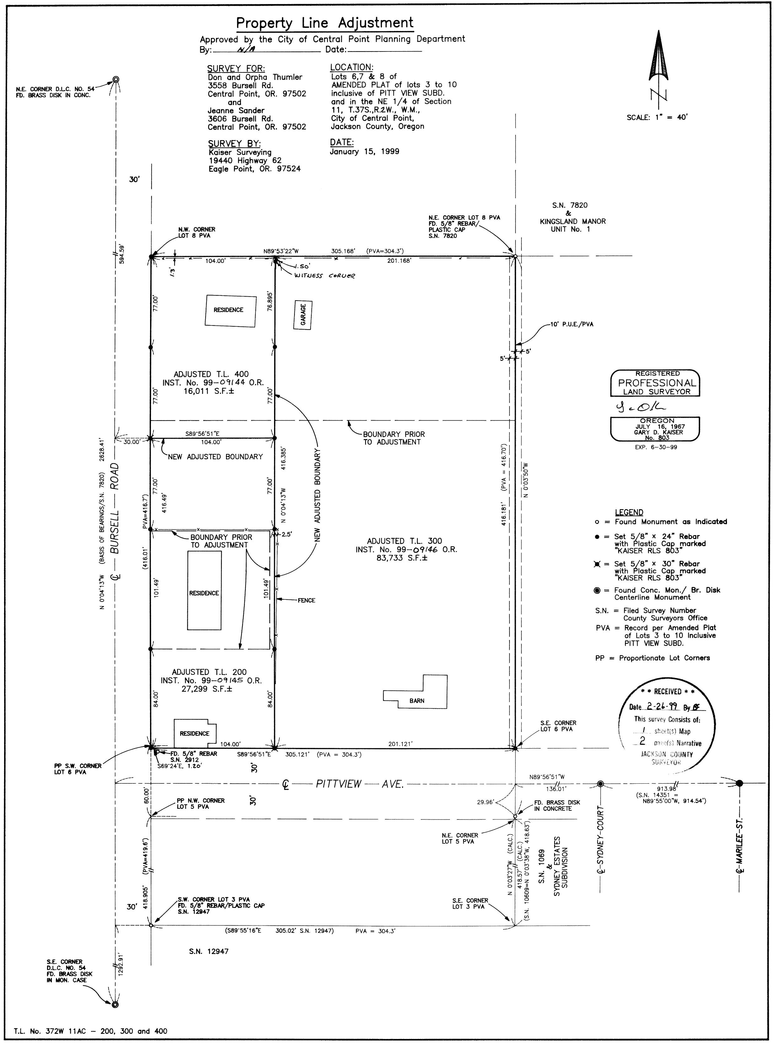
Bursell Road (the East boundary of D.L.C. No. 54) that I develop overages on the North boundary of Lot 8, (measure 305.16811'), (PLAT=3'4.3') (calc. from SN 7820=304.27') and on the South boundary of Lot 6 (measure=305.121') (plat=304.3') (calc. from SN 7820=304.72').
