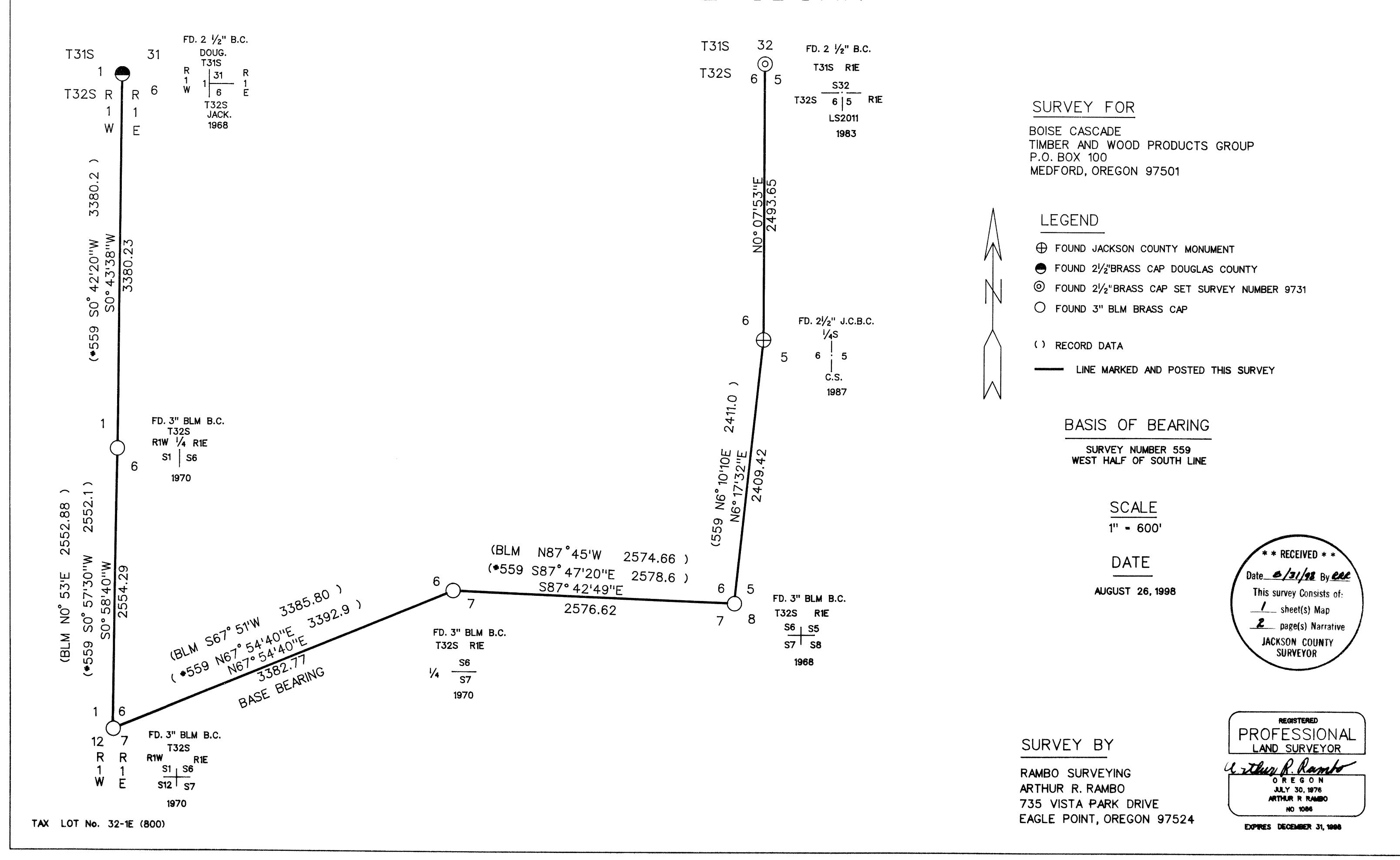
AT THE CLOSING SECTION CORNER COMMON TO SECTION 5 AND 6, TOWNSHIP 32 SOUTH, RANGE 1 EAST, AND SECTION 32, TOWNSHIP 31 SOUTH, RANGE 1 EAST I FOUND A 2 1/2" DIAMETER BRASS CAP SET SURVEY NUMBER 9731.
