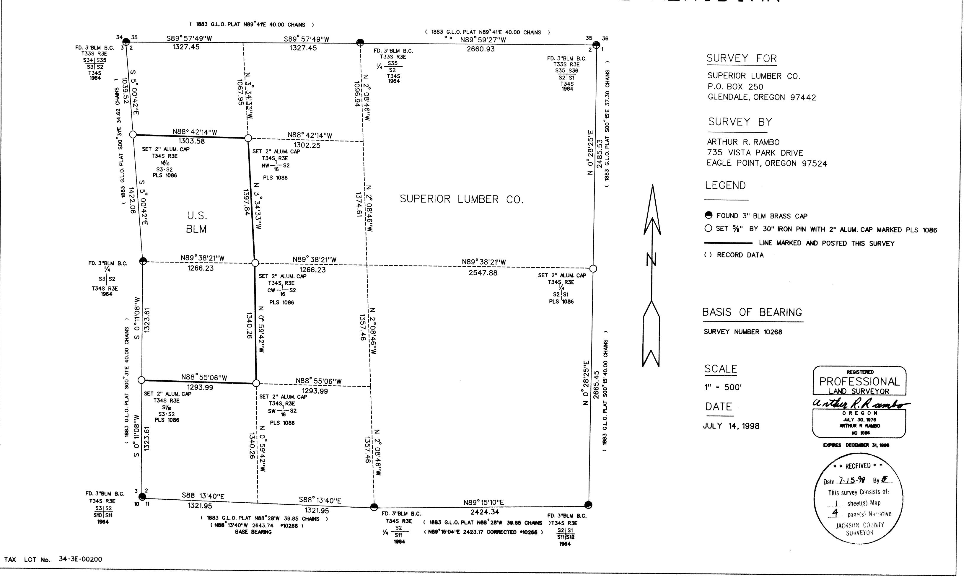
SOUTH ONE-SIXTEENTH CORNER COMMON TO SECTION 2 AND SECTION 3 TOWNSHIP 34 SOUTH RANGE 3 EAST. AT THE CORNER POINT I SET A 5/8" BY 30" IRON PIN WITH A 2" DIAMETER ALUM. CAP MARKED:
